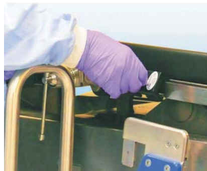
Photo 4 Attaching the Rail Clamp to the Rail
