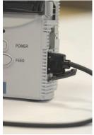
**Printout** – Once the printer is operational and the cables are in place, the LifeDop will automatically download the waveform and printing will begin. If the PRINT button is pressed while the printer is connected and ready, printing will start immediately.
