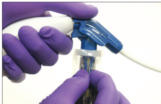
Photo 9 Removing the Adapter Drape from the ALLY UPS® Arm
