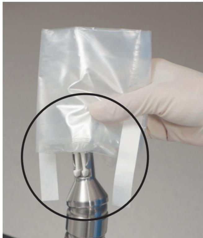
**Photo 3b** Pinch Clips in the Seated Position
