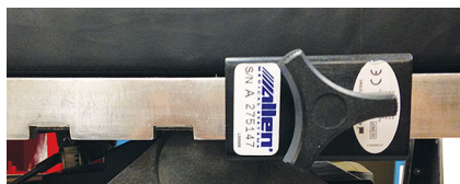
Figure 2b: Move the clamp to the right, away from the slots in the rail
