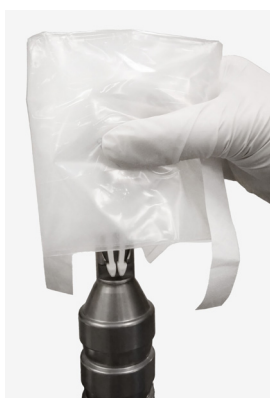
Figure 3b: Final position of the adapter drape in the connector
