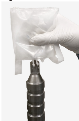
Figure 3a: Holding the sterile adapter drape
