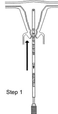
8. While one hand holds the device sheath in place, withdraw the piston rod with the other hand.
