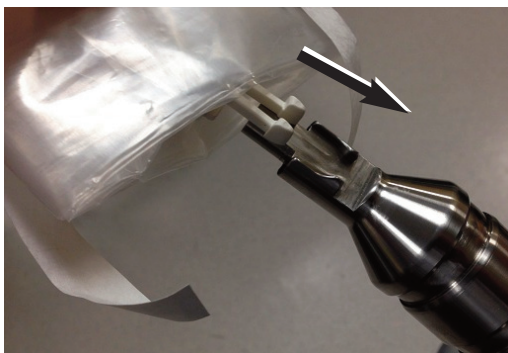
Photo 3a Installing the Adapter Drape with the Pinch Clips
