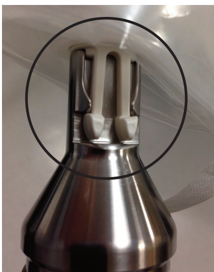
Photo 3b Pinch Clips in the Seated Position
