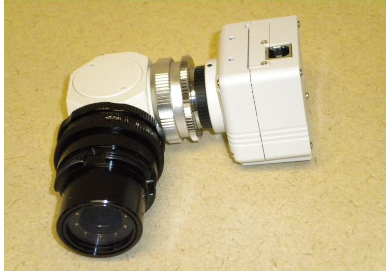
3. Then attach the C-Mount Adaptor to the TriScope.
