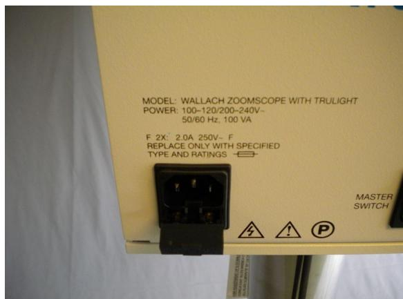
3. To remove, pull out the drawer beneath the power socket.
