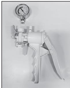
2. Remove the pump gauge by turning the gauge counterclockwise while supporting the pump junction
