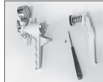
1. Remove the pump handle by using a screw driver while supporting the pump junction
