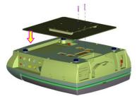
2 Turn the monitor over. Lift it and slide the adapter plate into the groove of the top splint sideways. When the board goes halfway, pull down the pin on the back of the top splint to allow the board to go through. Keep pushing the board in until the pin rebounds and clicks into the hole. The edges of the adapter plate and the top splint should match perfectly at this time.
